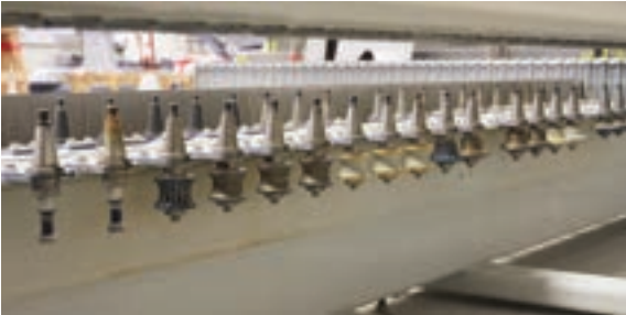
Multiple sets of tools mounted on cones in sequence to be used
